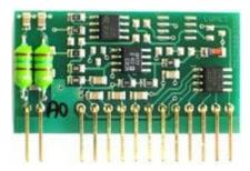
Accuracy -50 to 100°C  $\pm 0.2$ °C 100 to 250°C  $\pm 0.2$ % from reading. Galvanically unisolated. Two-wire connection.
