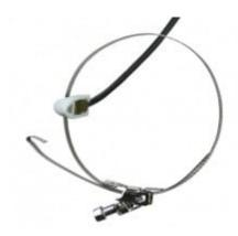
Temperature probe with Pt1000 sensor. Surface probe for tubing and flat surface, range from -30 to +130 $^{\circ}$ C, 2 meters cable, IP65. With ELKA connector.
