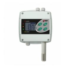
Humidistat, thermostat with two relay outputs. Outdoor, indoor use. Built-in humidity, temperature sensors. Measured values are also converted to other humidity interpretation: dew point temperature, absolute humidity, specific humidity, mixing ratio, specific enthalpy.
