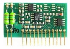
$\label{eq:constraint} \mbox{Accuracy $\pm 0.1\%$ FS. Galvanically unisolated.} \\ \mbox{Two-wire connection.}$
