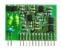
Thermocouple K (NiCr-Ni) input. Measuring range -70 to +1300°C. Accuracy  $\pm 0.3\%$  from reading + 1.5°C. Linearized, cold junction compensation. Galvanically unisolated.
