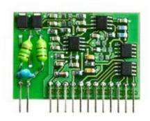
Thermocouple S (Pt10%Rh-Pt) input. Measuring range 0 to  $+1700^{\circ}$ C. Accuracy  $\pm 0.3\%$  from reading  $+1.5^{\circ}$ C from +200 to  $+1700^{\circ}$ C. Linearized, cold junction compensation. Galvanically unisolated.
