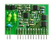
Thermocouple B (Pt30%Rh-Pt) input. Measuring range +100 to +1800°C. Accuracy  $\pm 0.3\%$  from reading +1.0°C from +300 to +1800°C. Linearized, without cold junction compensation. Galvanically unisolated.
