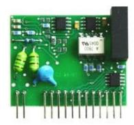
Accuracy -50 to  $100^{\circ}\text{C} \pm 0.2^{\circ}\text{C}$  100 to  $250^{\circ}\text{C} \pm 0.2\%$  from reading. Galvanic isolation is not designed as safety protection.
