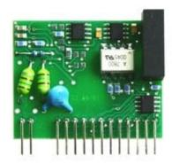
Accuracy -140 to+100°C  $\pm 0.2$ °C 100 to 600°C  $\pm 0.2$ % from reading. Galvanic isolation is not designed as safety protection.
