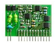
Thermocouple T (Cu-CuNi) input. Measuring range -200 to +400°C. Accuracy  $\pm 0.3\%$  from reading + 1.5°C. Linearized, cold junction compensation. Galvanically unisolated.
