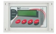
Terminal with dual line alphanumerical LCD and control buttons, audio alarm indication and 32 alarm LEDs - for panel mounting or mounting to a case lid. Identical functions as built-in terminal of MS data logger. It is possible to build in with IP54 protection. Maximum cable length to data logger 50m. It is necessary to order the MP017 connection cable to data logger.
