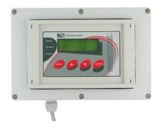
External terminal with dual line alphanumerical LCD, control buttons, 32 alarm LEDs and audio alarm indication. Built in a IP54 protection case, including 2m cable with covered terminals. Identical functions as built-in terminal of MS5D data logger. Maximum cable length to data logger 50m
