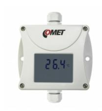
Temperature transmitter for Pt1000/3850ppm sensor with 4-20mA output for two-wire connection is built in a durable watertight case. Output temperature range is user adjustable. Degrees Celsius and Fahrenheit are user selectable.
