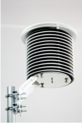
Professional passive solar radiation shield for better protection of weather sensors and barometers and for more accurate measurement, naturally ventilated.
