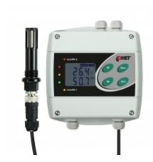
Humidistat, thermostat with two relay outputs. T+RH probe from hard anodized duralumin for compressed air up to 25 bars with 1 meter cable. Outdoor, indoor use.
