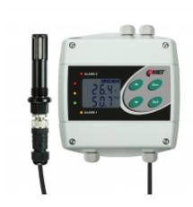
Humidistat, thermostat with two relay outputs. T+RH probe from hard anodized duralumin for compressed air up to 25 bars with 4 meters cable. Outdoor, indoor use.
