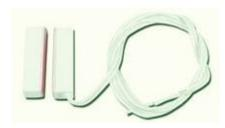
Magnetic door contact, connectable to binary inputs with cable length 20 meters. Plastic body. The dimensions of 49x14x13mm, working distance of 30 mm
