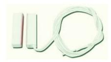
Magnetic door contact, connectable to binary inputs with cable length 30 meters. Plastic body. The dimensions of 49x14x13mm, working distance of 30 mm.
