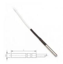
Multi-purpose watertight IP67 probe -190 to  $+150^{\circ}$ C. Accuracy class B. Stainless steel 17240 with teflon cable of specified length, with ELKA connector. Diameter 5  $\pm$  0.1 mm, length 50mm.
