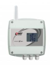
The transmitter measures the temperature from three external K-type thermocouple probes (NiCr-Ni) and the ambient temperature using a built-in sensor..
