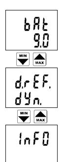
Battery voltage of partially loaded battery is displayed. This value illustrates battery condition.
