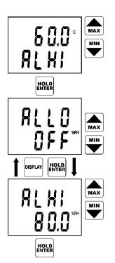
Reading ALHI indicates adjusted upper limit of the same alarm (here air temperature). Set the desired value in the same way as in above lower limit. If needed it is possible to get back to lower limit setting of the same alarm by pressing DISPLAY key. Press ENTER key to confirm new upper limit.
