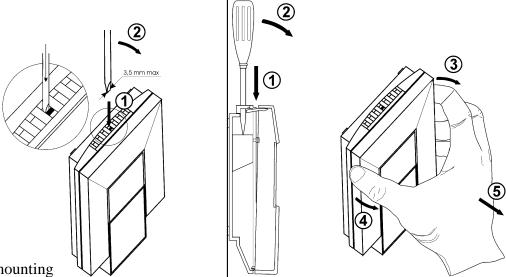
Figure 2: Device demounting
