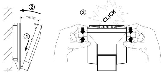
Figure 1: Device mounting
