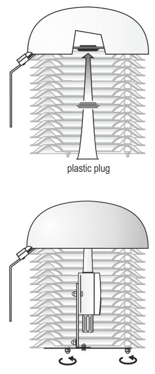
7 - place the assembly of cover plate and holder FP001 with the IoT sensor in the radiation shield in the position as shown
