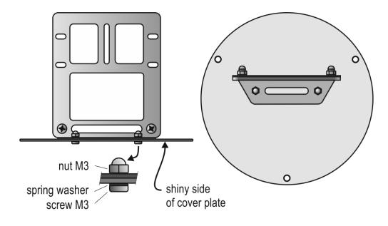
3 - fasten the FP001 holder to the cover plate with two M3 screws in the position as shown
