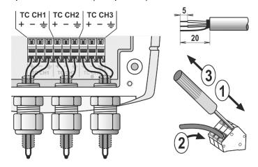
Finally, tighten the cable glands of the connected thermocouple probes to secure and seal the cables. Cables / wires with a diameter of less than 2 mm cannot be sealed in the gland. Also, do not use probes with a braided jacket (glass or metal fabric) in applications where you require the device to be waterproof. Insert attached plug into unused cable glands to seal the device.
